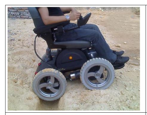
Special design PU solid tire: Hard-wearing (Rubber tire available-strong traction)
